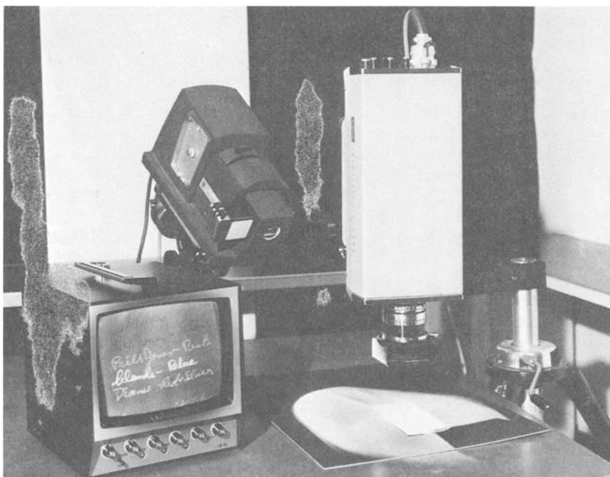
FIG. 2—Camera, monitor and mercury vapor light source.
